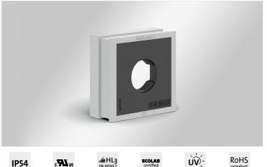
QT-AT-M is an adapter grommet (based on large QT grommets) with integrated metric threads.. The QT-AT-M adapter grommets are made of elastomer with a polyamide body. QT-AT-M adapter grommets are available with inner threads M12 x 1.0, M16 x 1.5, M20 x 1.5 and M25 x 1.5.
